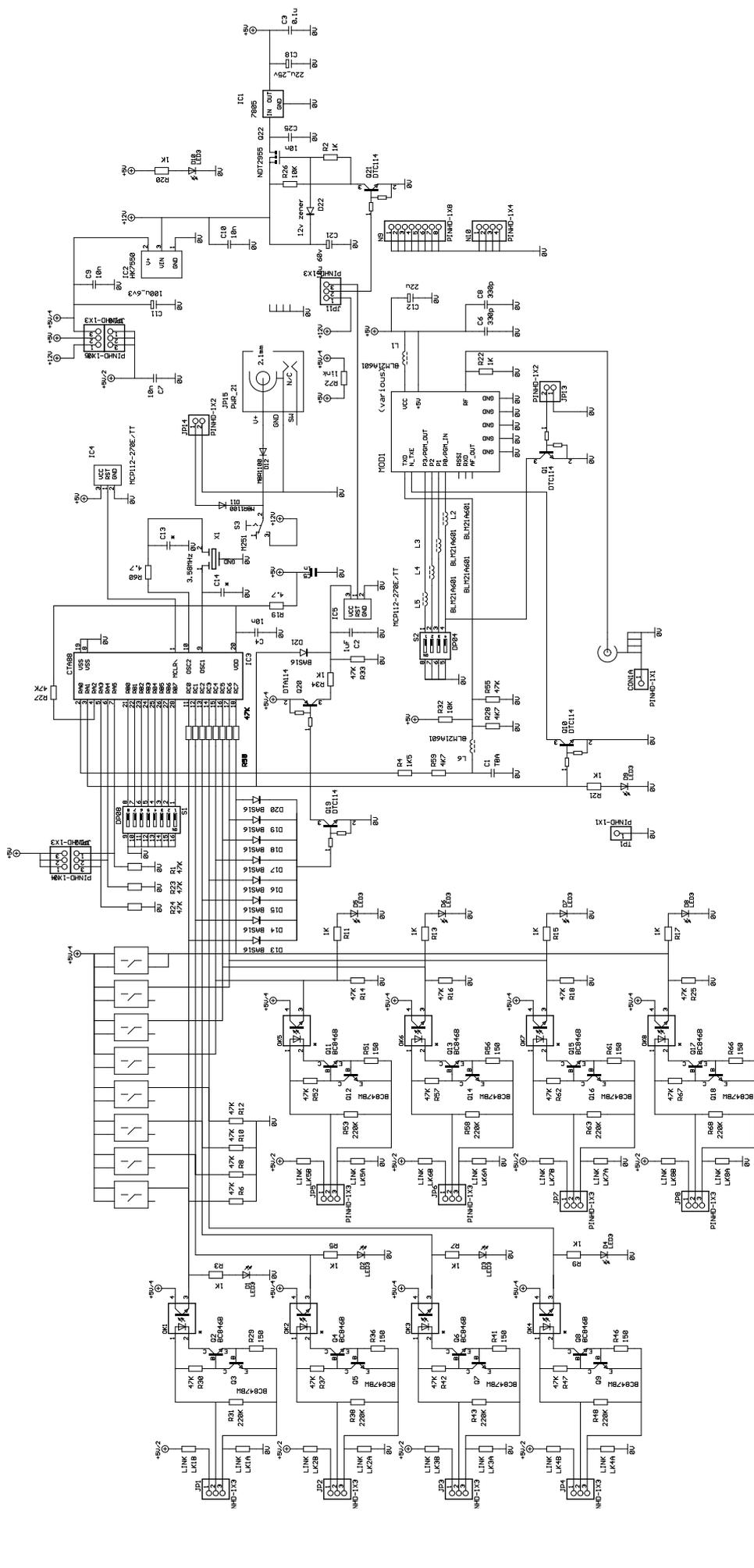
Figure 9: Schematic of CTA88 Encoder application board for SHX1T / UHX1T / FPX33T Transmitter
