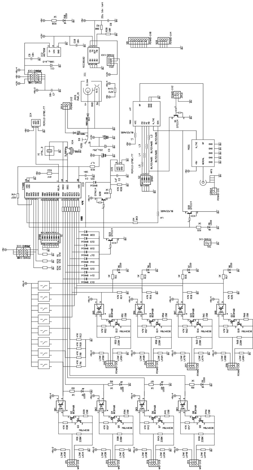
Figure 7: Schematic of CTA888H Encoder application board for AFS2 Amplifier, LMT2 Transmitter
