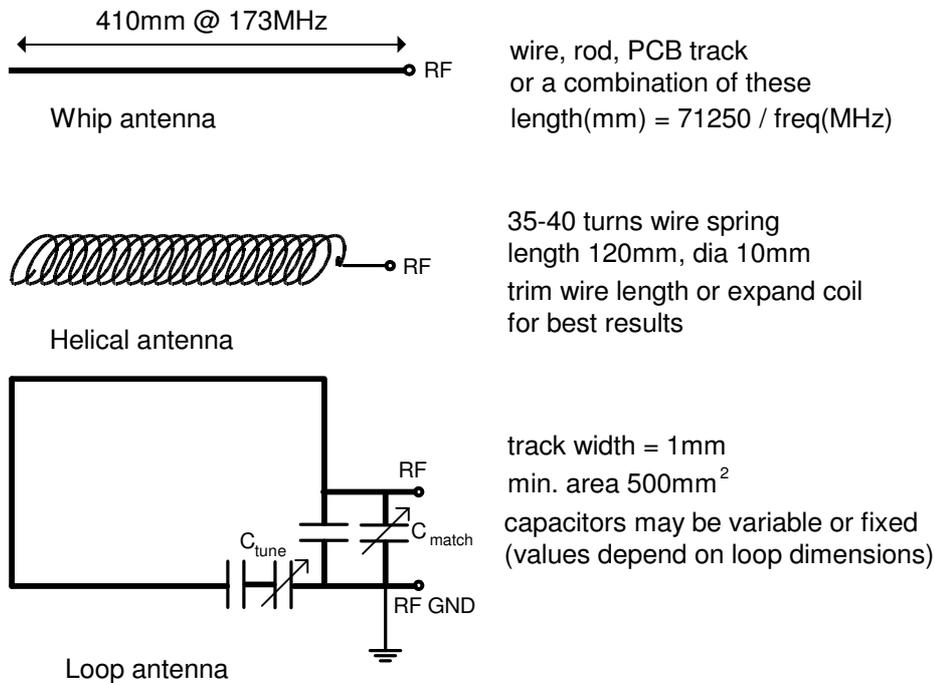
Figure 5: integral antenna configurations
