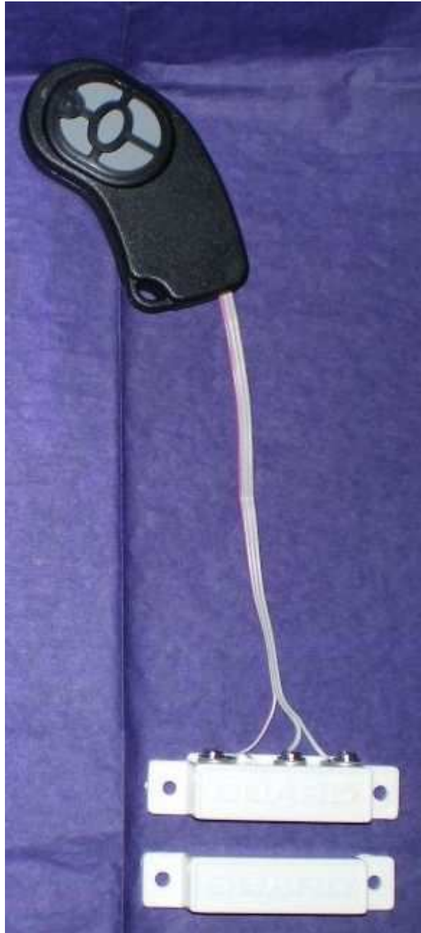
Fig. 6: KFX2 keyfob (external) connected to reed switch with magnet shown
