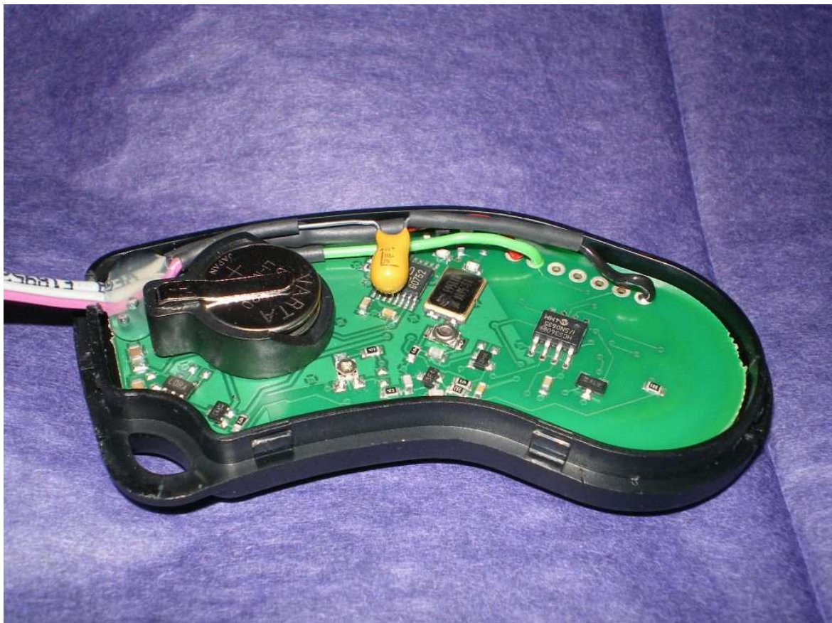
Fig. 5: KFX2 keyfob (internal) shown with additional resistor and capacitor
