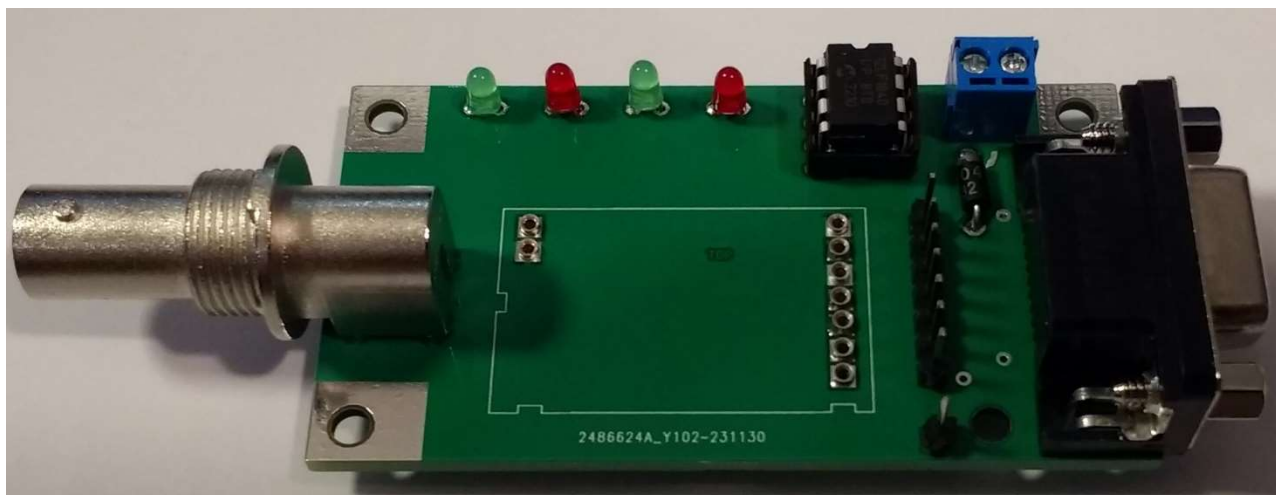
Figure 3: CNM2/CNM3 Evaluation Kit with RS232 interface and bus activity LEDs
