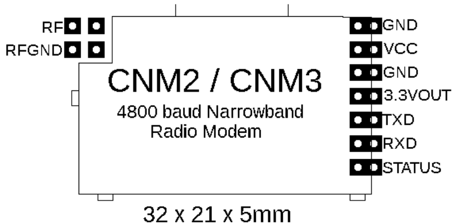
Figure 2: CNM2/CNM3 Pinout and Dimensions
