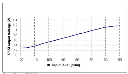
Fig.4: Typical RSSI response curve
