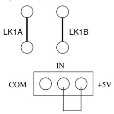
LK1A will link the COM to the system ground LK1B will link the +5V to the +5V system rail.
