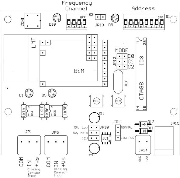
Figure 2: CTA28 TX application board PCB (top view)
