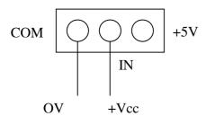
**COM**: Local ground (not connected to system ground)
