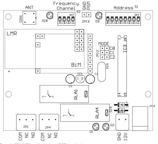
Figure 3: CTA28 RX application board PCB (top view)
