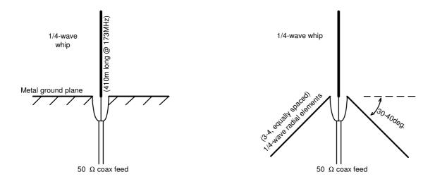
Figure 6: Quarter wave antenna / ground plane configurations
