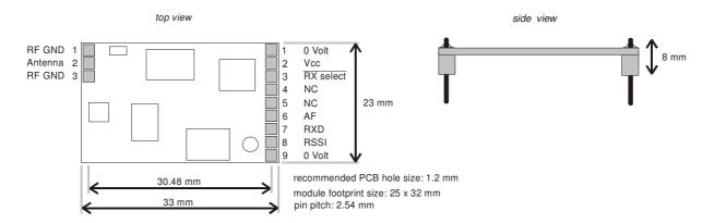
Figure 3: Pin-out and dimension
