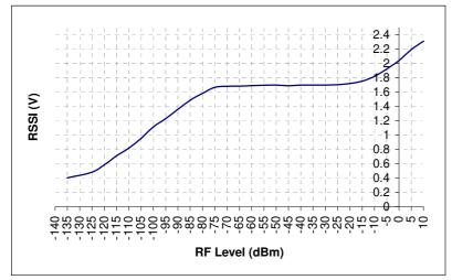
Figure 4: RSSI level with respect to received RF level at CVR1 antenna pin
