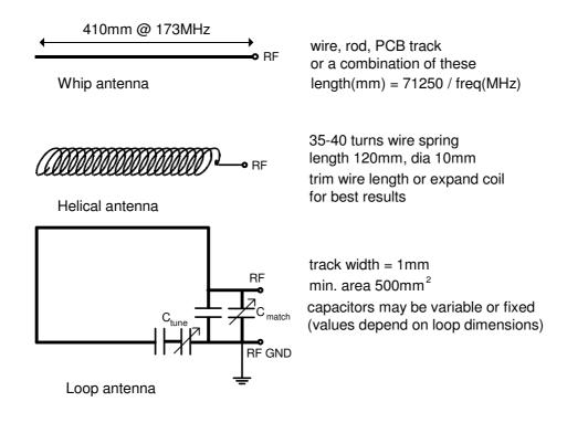
Figure 5: integral antenna configurations
