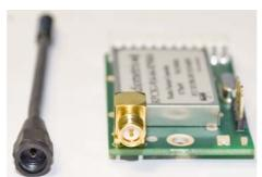
Fig 19: 914MHz 1/4 wavelength monopole antenna with Reverse Polairy SMA connector (ANT-914-W-RPSMA)
