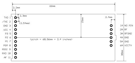
Figure 3: SHX1 footprint (Top) view
