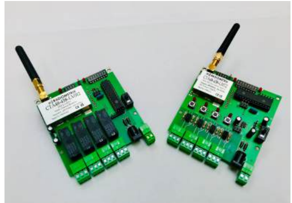
Figure 1: CTA48 application boards
