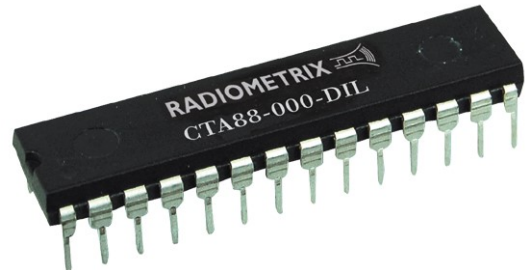
Figure 1: CTA88A in 28 pin DIL package
